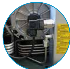
Pressure switch for automatic stop
