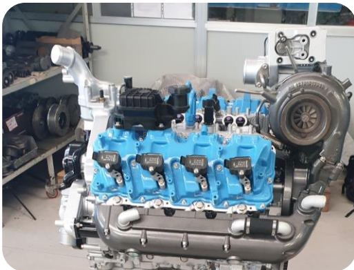
V8 Engine during assembling phase in Italtecnica
